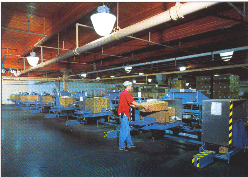
From the mezzanine, case bottoms are provided to the production area below from nine SIMS ER-1600 Case Erectoring Machines with bottom sealers.
